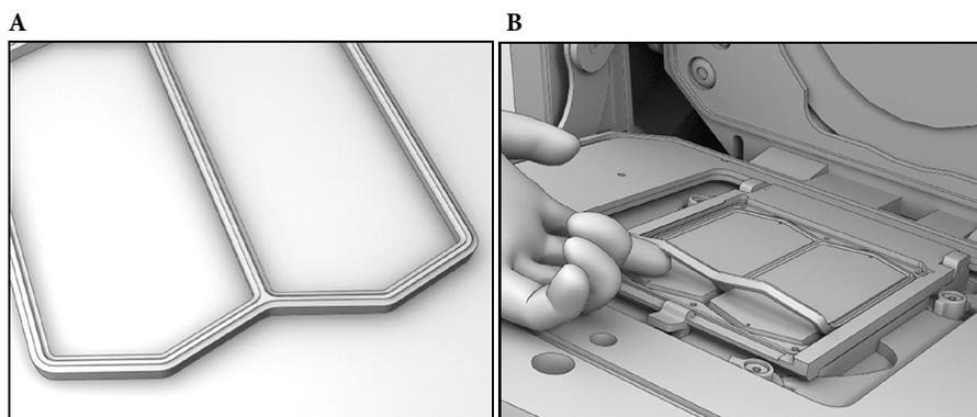
Figure 30: Orientation and placement of the cartridge seal
