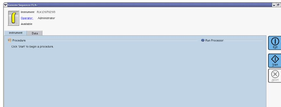
Figure 19: Upper portion of the GS Sequencer software main window, with the Instrument tab active
