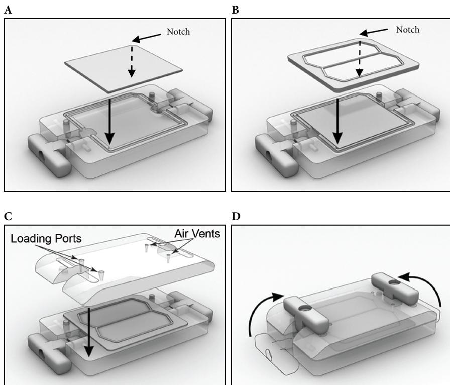
Figure 9: Assembly of the Bead Deposition Device
