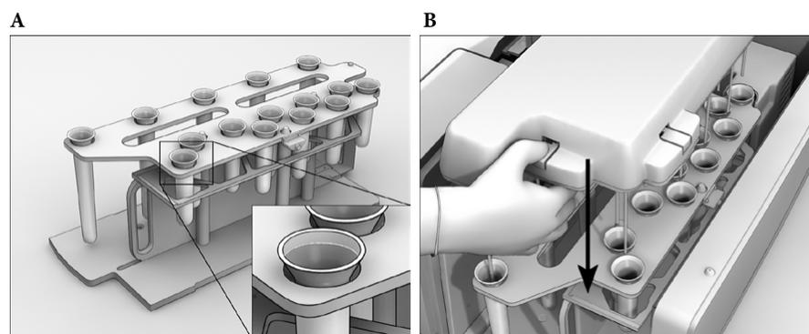
Figure 5: Filling the Pre-wash Tubes; loading before a pre-wash
