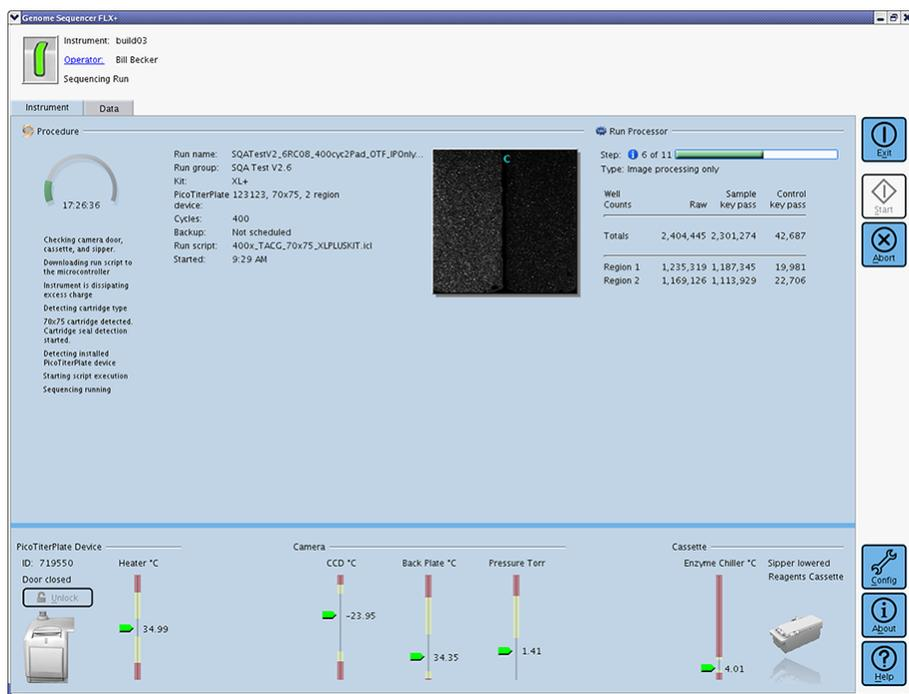
Figure 32: The Instrument tab of the GS Sequencer application main window during a sequencing Run
