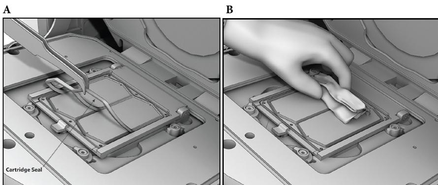
Figure 18: Removing the PTP cartridge seal and wiping the PTP cartridge
