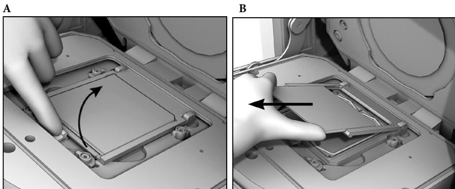
Figure 17: Removing the used PicoTiterPlate device
