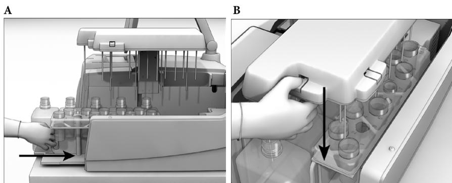
Figure 14: Loading the Reagents Cassette into the instrument
