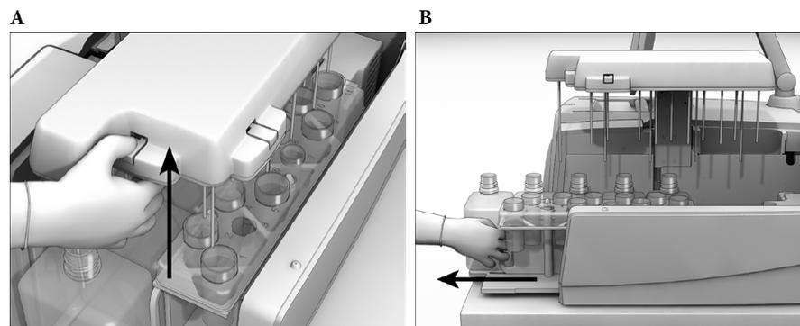
Figure 4: Removing the GS FLX+ Reagents Cassette (from the previous Run)
