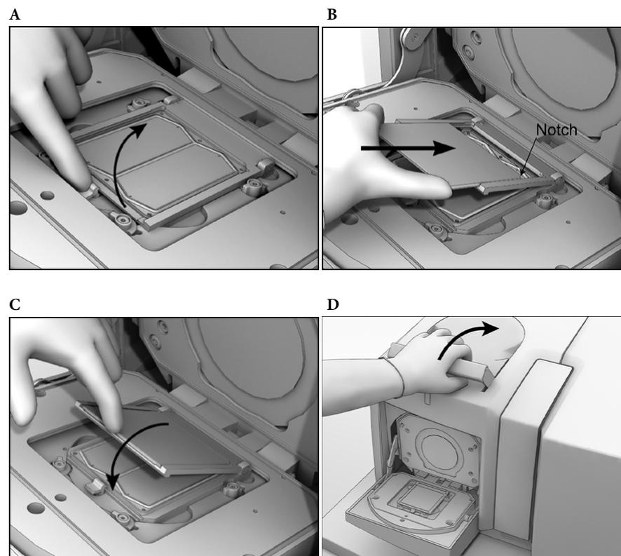
Figure 31: Loading a PTP device into the PTP frame, in the cartridge
