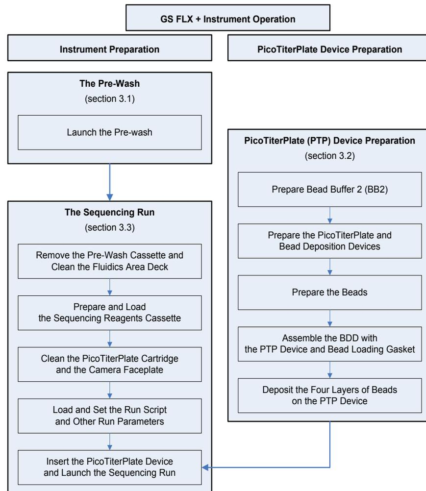
**Figure 1: Workflow of a sequencing Run performed on the GS FLX+ Instrument, with the GS FLX Titanium Sequencing Kit XL+**
