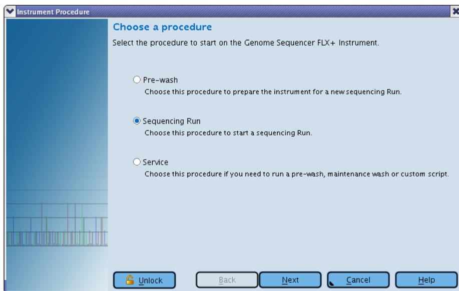
Figure 20: The Run Wizard's first window: Choose a procedure, with Sequencing Run option selected
