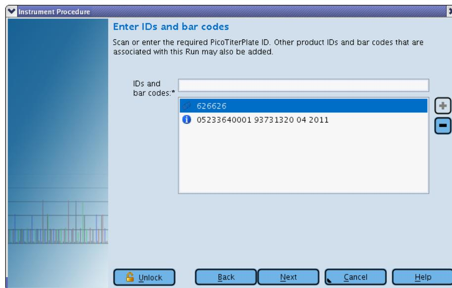
Figure 21: The Run Wizard's second window: Enter IDs and bar codes
