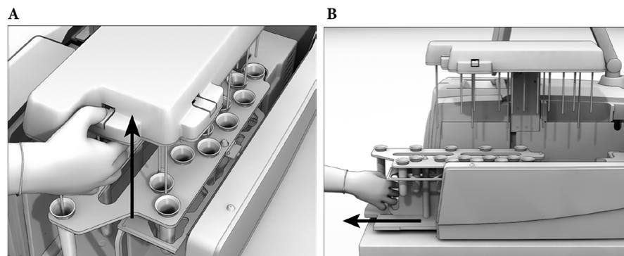
**Figure 11: Removing the Pre-wash cassette from the instrument**
