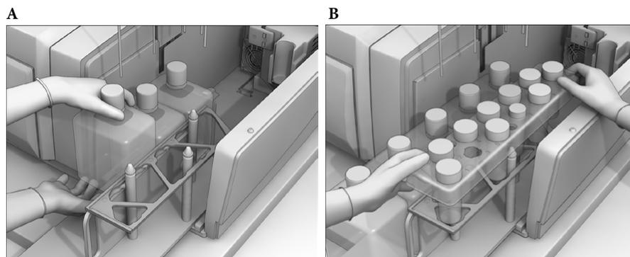
Figure 13: The Sequencing Reagents tray in the proper orientation
