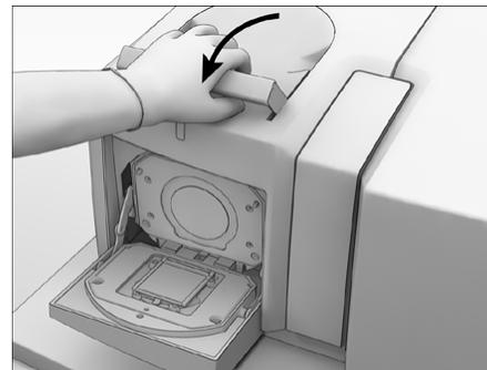
Figure 16: Opening the camera door
