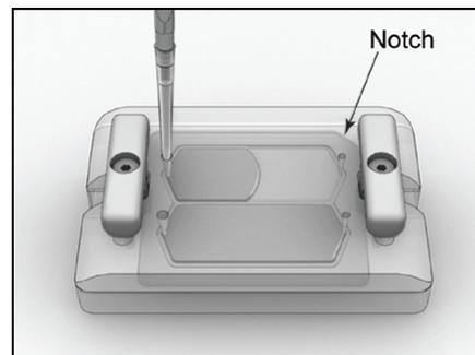
**Figure 10: Filling the loading regions of the assembled Bead Deposition Device**
