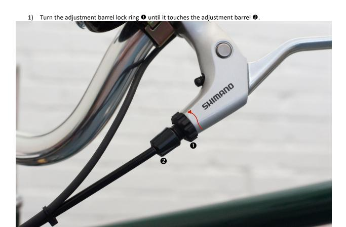
2) Turn the adjustment barrel until the lock ring bottoms out on the lever housing.
