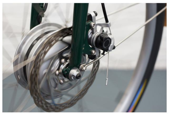
6) With a 3mm hex key, turn the inner pad adjustment clockwise 1 click (1/6<sup>th</sup> of a turn in direction of arrow).
