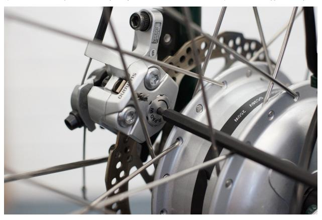
4) With a 2.5mm hex key, turn the outer pad adjustment screw 2 turns counterclockwise (make the screw stick out more)
