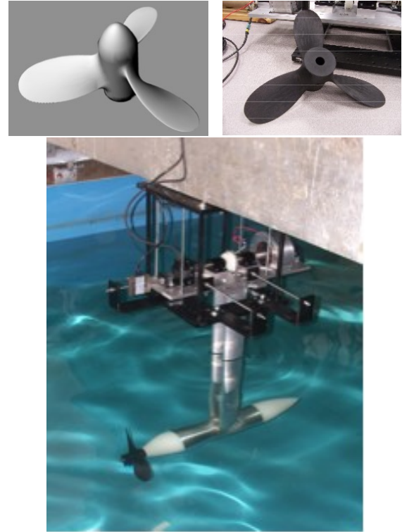
Figure 11. OpenProp rendering, 3D printed model, and tow-tank testing of propeller OP4148.
