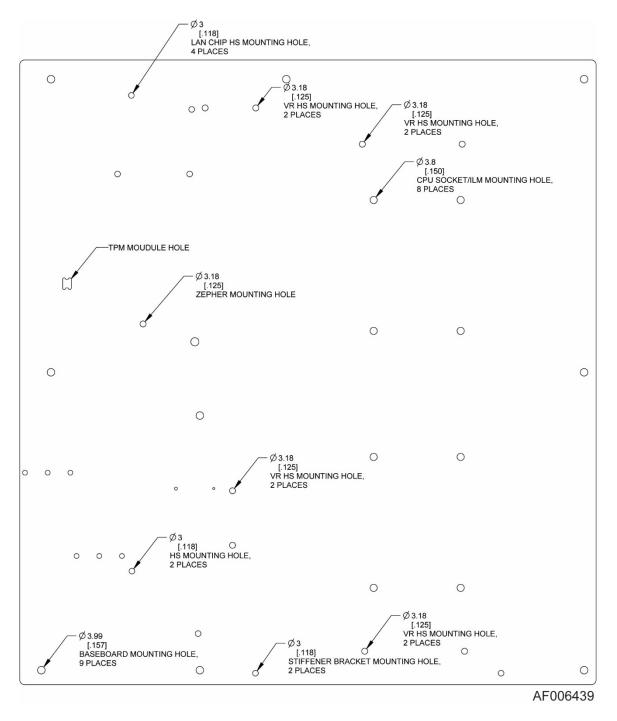
Figure 5. Mounting Hole Locations (2 of 2)
