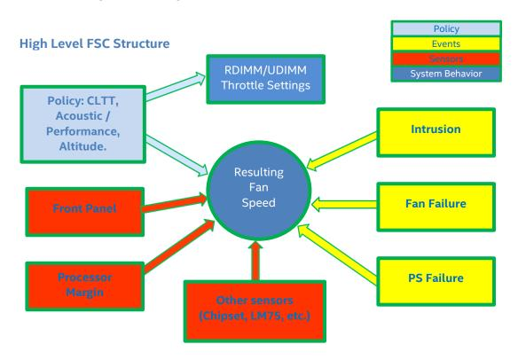
Figure 18. High-level Fan Speed Control Process
