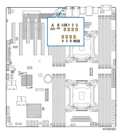
Figure 35. POST Code Diagnostic LED Decoder
