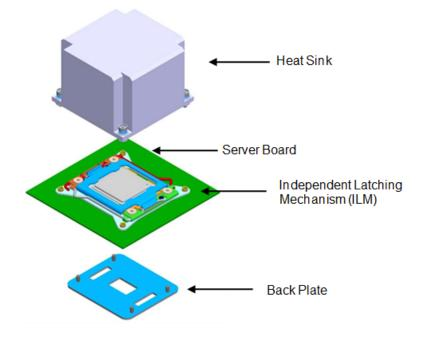
Figure 13. Processor Socket Assembly
