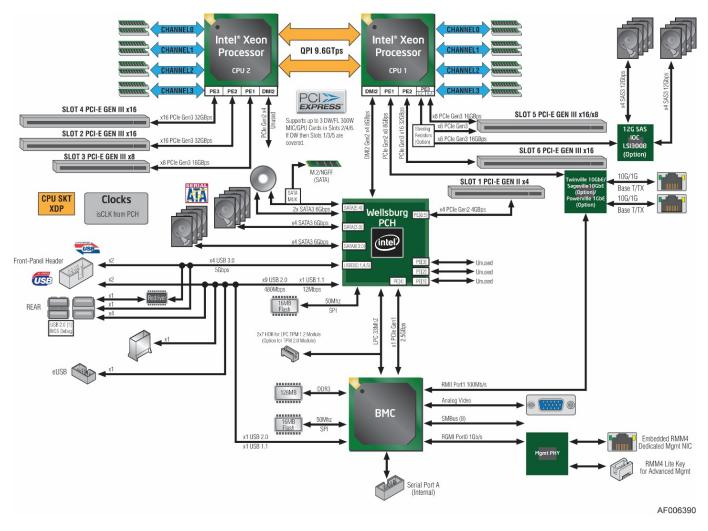
Figure 12. Intel® Server Board S2600CW2SR/S2600CWTSR Functional Block Diagram
