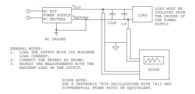
Note: When performing this test, the probe clips and capacitors should be located close to the load.
