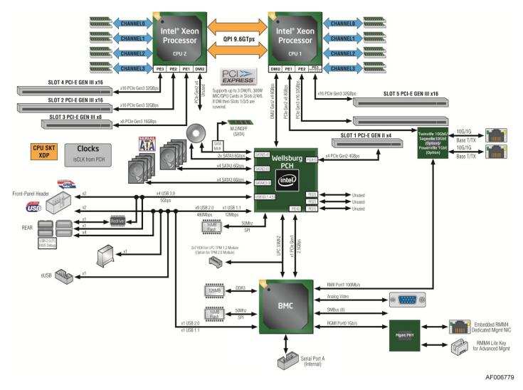
Figure 11. Intel® Server Board S2600CW2R/S2600CWTR Functional Block Diagram
