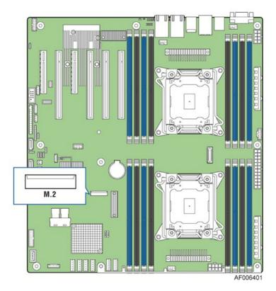
The following diagram shows how the M.2/NGFF modules are installed on the connector.
