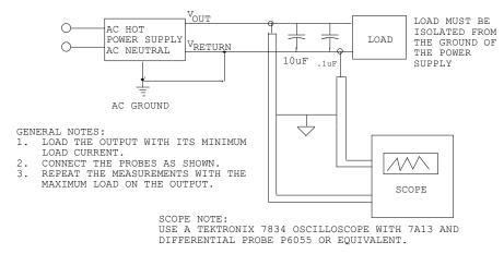
Figure 27. Differential Noise Test Setup
