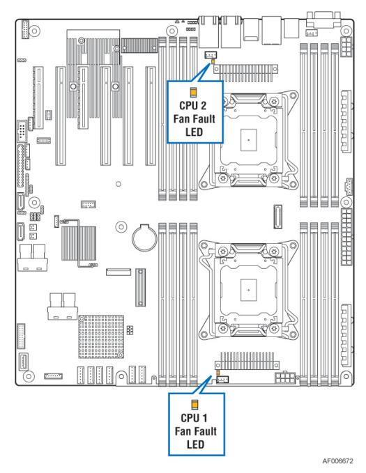
Figure 23. Fan Fault LED's Location
