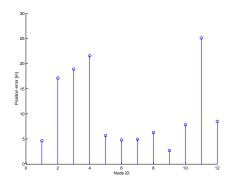
Fig. 11. The localization error for each of the unknown nodes when using multilateration.
