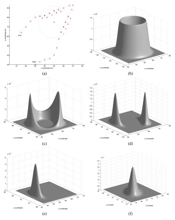
Fig. 6. (a) The trajectory of the mobile beacon and the position of the nine beacon transmissions received by the unknown node. (b-f) The evolution of the position estimates of the unknown node after 1,2,4,5 and respectively 9 beacon packets have been received.
