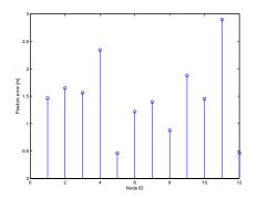
Fig. 9. The localization error for each of the unknown nodes when using the proposed probabilistic approach.
