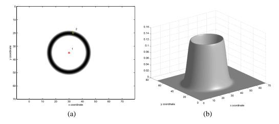
Fig. 5. (a)The constraint imposed on the position of the unknown node 2 when a beacon packet of coordinates (30,35) and RSSI 75 is received from the mobile beacon 1; (b) A 3D view of the constraint.
