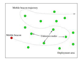
Fig. 4. One mobile beacon assisting in the localization of a sensor field.
