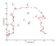
Fig. 7. The real (denoted by an 'o') and the estimated (denoted by an 'x') positions of the unknown nodes and the trajectory of the mobile beacon used in the experimental setup.
