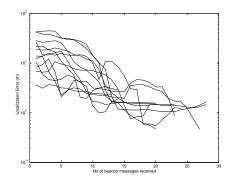
Fig. 10. Evolution of the localization error with the number of beacons received.
