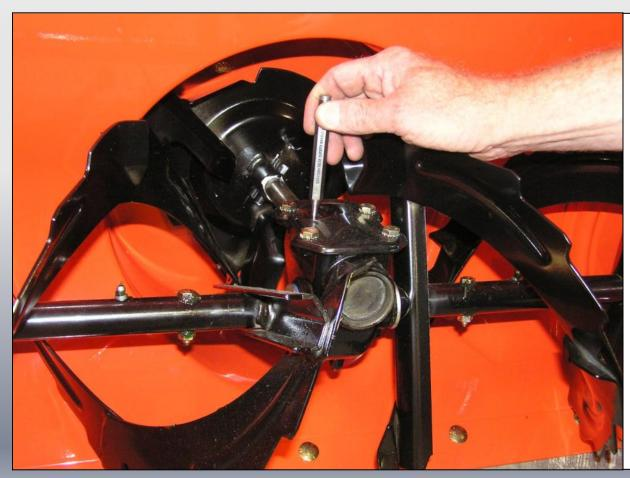
Check oil level in auger gearcase (see *Check Auger Gearcase* in Owners Manual).
