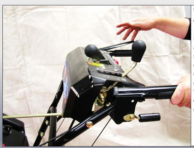
With power switch in the off position, press down (engage) both clutch levers. Release attachment clutch (right side) lever. Attachment clutch should remain engaged until traction clutch lever is released, then both clutches *must* disengage. If they do not, contact your dealer for repairs.
