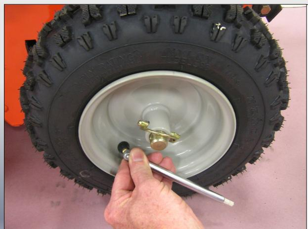
Check tire pressure and adjust to the pressure listed on tire sidewall.
