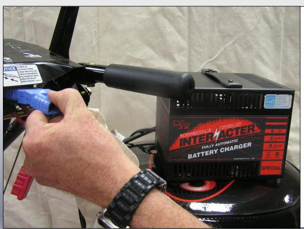
The batteries MUST be charged for a minimum of 7 hours before the first use. See *Pre-Start* in Owners Manual.
