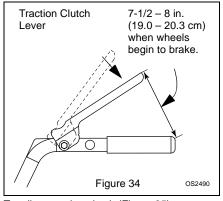
To adjust traction clutch (Figure 35):
