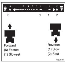
**IMPORTANT:** DO NOT change motion from forward to reverse with clutch engaged. Forward speed can be changed without declutching.
