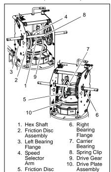
Insert new friction disc assembly into frame. Install washers onto carrier bearing and slide into speed selector arm.
