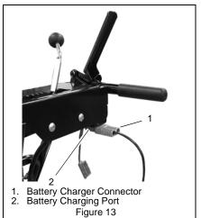
Plug battery charger into wall outlet. Do not use an extension cord unless necessary. If an extension cord is needed follow the manufacturer's recommendations for length and capacity.
