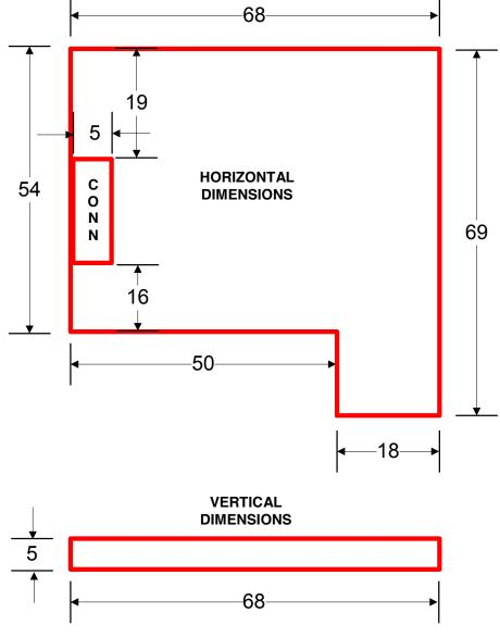
Figure 2. Internal Flexspace Dimensions
