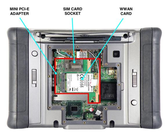
Figure 1. Rear Compartment Flexspace
