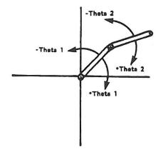
Figure 5-11. Movement in Joint Frame
