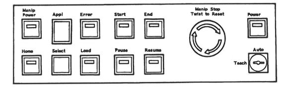
Figure 5-7. Servo Power Module Operator Control Panel
