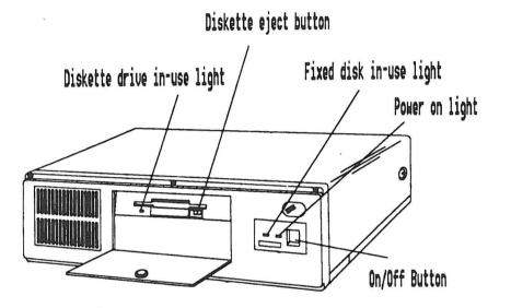
Figure 5-6. 7537 Controls and Indicator Lights
