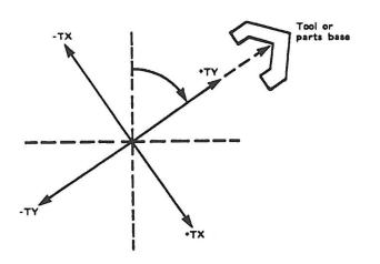
Figure 5-13. Movement in Tool Frame
