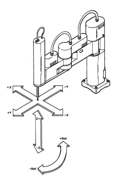
The manipulator tool shaft moves horizontally on a jointed arm. This horizontal movement is defined as being in an X and Y plane.
