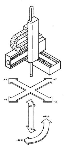
Figure 5-5. CCR Manipulator Movement
