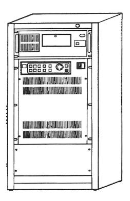
Figure 5-2. Controller and Servo Power Module Mounted in a 19-Inch Rack
