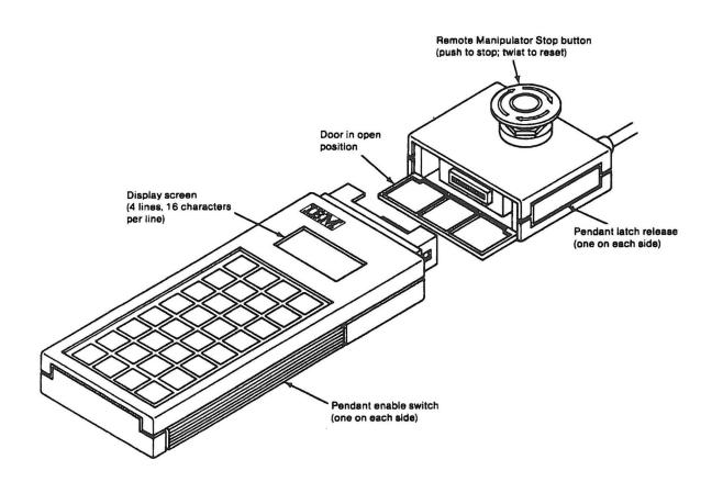
Figure 5-8. Pendant Being Connected to the Remote Manip Stop Button
