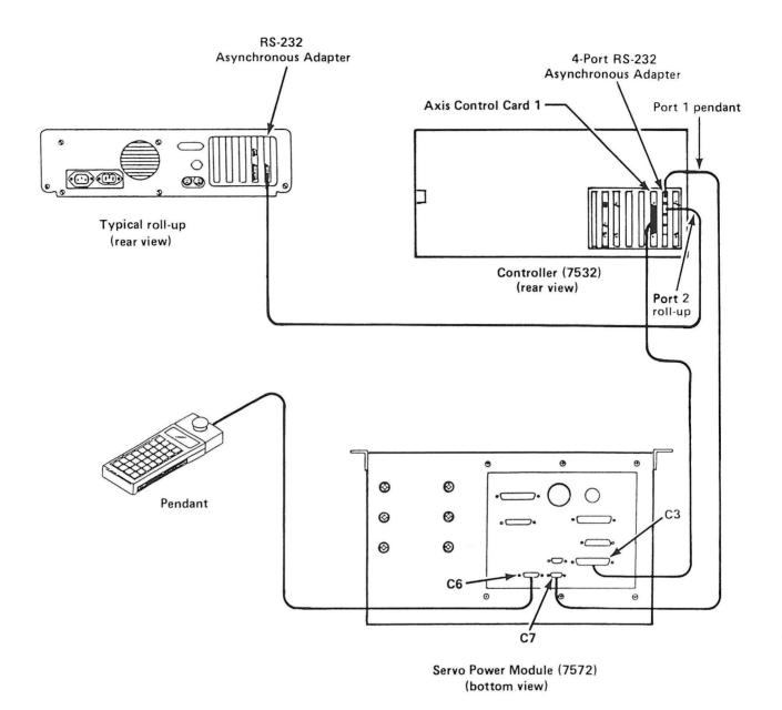
Figure 1-3. System Connections
