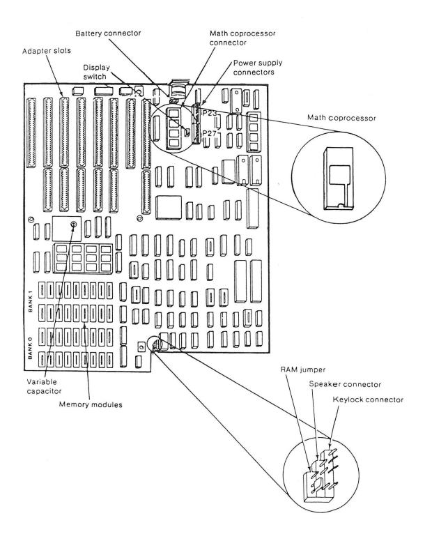
Note: The figure above shows four rows of memory modules with nine modules per row. Some 7532 system boards contain only two rows of memory modules with nine modules per row.
