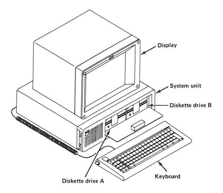
Figure 1-2. Roll-up Computer with Two Diskette Drives Installed
