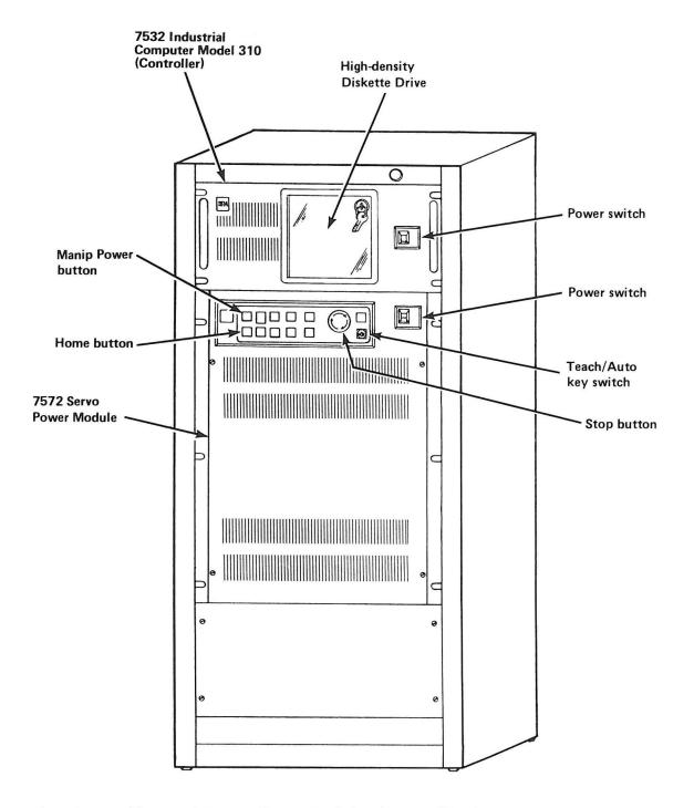
Figure 1-4. Controller and Servo Power Module (Front View)
