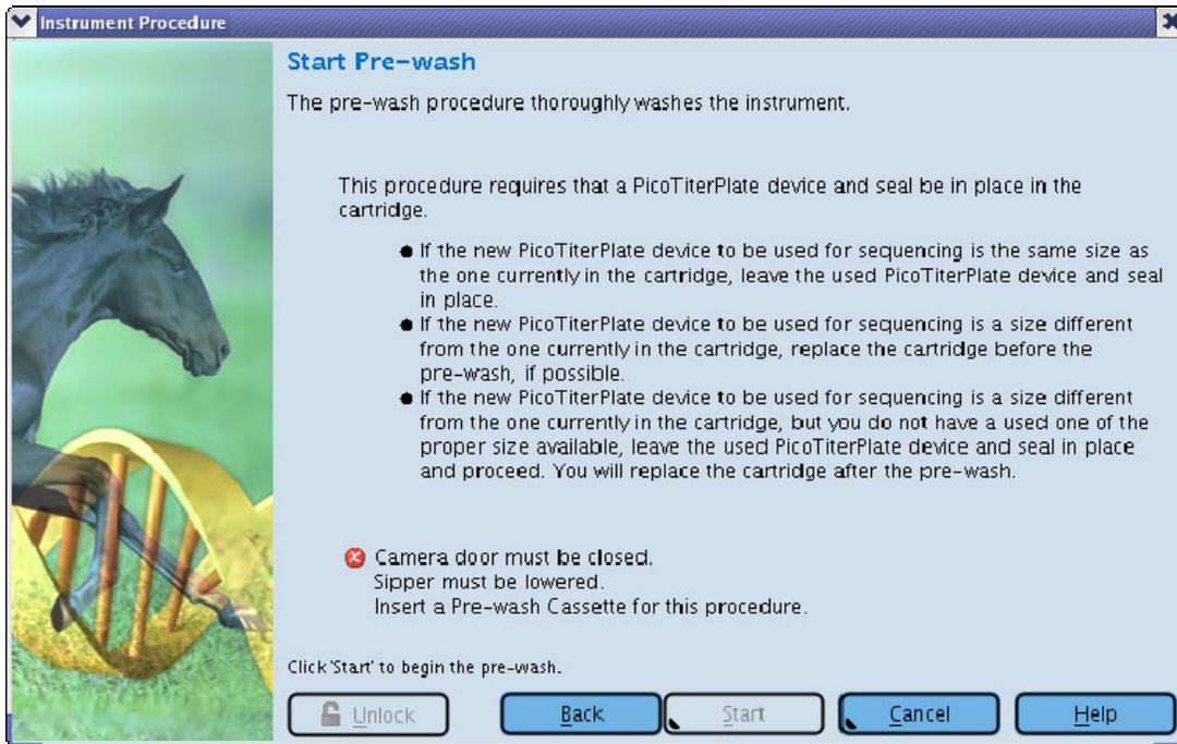
Figure 20: GS Sequencer Run Wizard – ‘Start Pre-wash’ window
